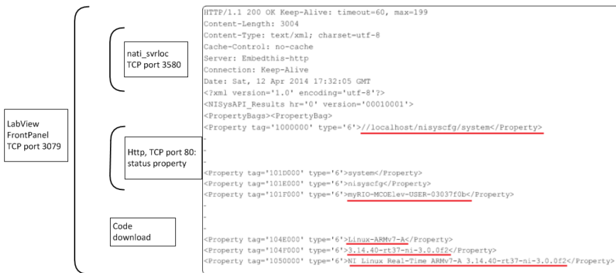
Figure 7. Communication history between LabVIEW and MyRIO. The underlined contents contain sensitive information of the equipment.
