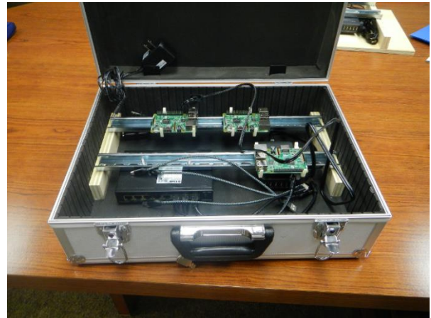
Fig. 1. Photo showing the completed CLIB. The case is an inexpensive aluminum "briefcase" with a foam lining adhered to the inside. Rails are mounted to plywood blocks glued to the inside of the case. Pis are mounted in clips to the tops of the rails. The switch and USB power supply are mounted to the bottom of the rails using screws and zip-ties. This leaves a small amount of space beneath the switch and power supply for network cables, power cords, the switch power supply and the power cord for the USB hub. There is also space for a portable monitor and keyboard (not shown) if desired.
