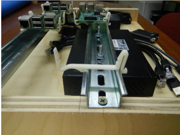
Fig. 2. Photo showing the prototype as well as the clips used to mount the Pis to the rails. The rails are commonly used to mount electrical devices such as controllers and relays to a backer board. A search on the Internet yields several sources for clips and holders that will mount Raspberry Pis to these and similar rails. The clips we chose were selected due to their minimal materials cost and ability to remain clear of all the Pi's ports and connectors. They also lent readily to unmounting and remounting the Pis.
